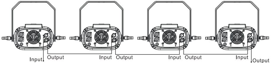
The number of daisy-chained fixtures is limited by the number of DMX channels required by the fixtures in relation to the maximum 512 channels available in one DMX universe. Note that if independent control of a fixture is required, it must have its own DMX channels. Fixtures that are required to behave identically can share the same DMX address and channels. To add more fixtures or groups of fixtures when the above limit is reached, add a DMX universe and another daisy-chained link.
